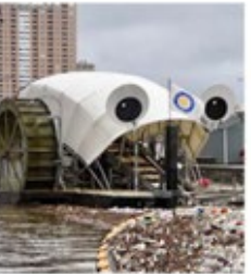
Trash Wheel Systems Typically installed on the side of a river, a water wheel powers a conveyor belt that brings trash from the water surface and into trash bins.
